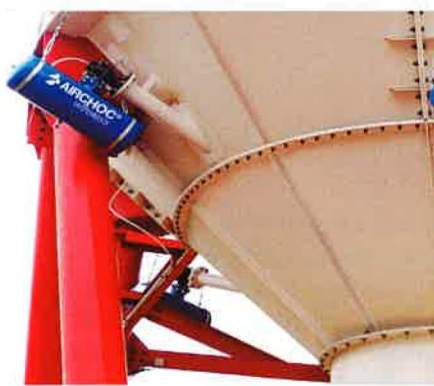
Figure 3. AIRCHOC® wireless on cement silo.
