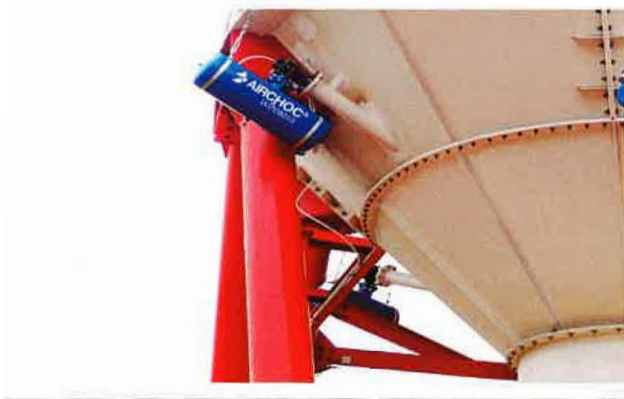
Figure 3. AIRCHOC® wireless on cement silo.
