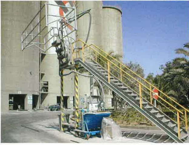
Figure 1. View of vacuuming installation for trailer cleaning.
