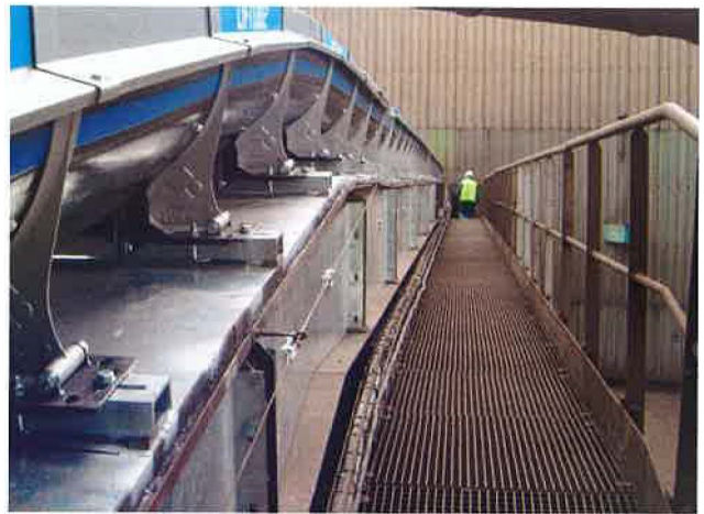
Figure 5. LIFTUBE® installation avoiding dust emissions.
