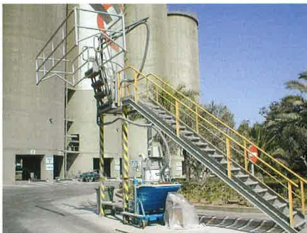
Figure 1. View of vacuuming installation for trailer cleaning.
